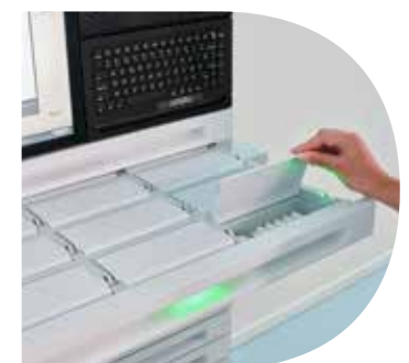
Smart Cart assigns a medication bin for each patient, opens bin for nurse to place all medications
